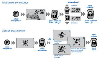
To switch off the control of warning or alarm zone by shock sensor, select s icon by pressing and select necessary mode with presses. Shortly press button to save settings.
