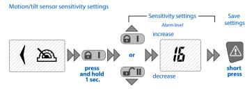
For prompt remote adjustment of alarm and warning levels of the motion/tilt sensor enter the settings menu, select (a) icon with (F III) button presses and press (a I) button for 1 second.
