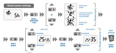
Short presses of FIII) button will switch between sensitivity settings of warning and alarm levels of the shock sensor. To save the new sensitivity values of the shock sensor, shortly press To exit this mode without saving, press and hold FIII) button for 1 second, otherwise it will end automatically in 10 seconds.
