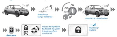
If you are planning to use remote and automatic engine start on a car with manual transmission, you will need to perform following actions before arming:
