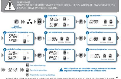
Automatic start and engine work conditions programming is done using LCD remote. Select (icon by pressing button and press button to enter remote start functions menu. This menu has 8 sub-levels that can be rotated by pressing (a). Sub-level values are changed using (b) and (c).
