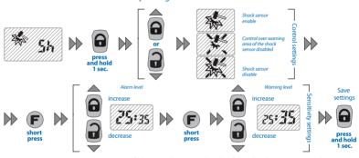
For prompt remote adjustment of alarm and warning levels of the shock sensor enter the settings menu, select so icon with button presses and press button for 1 second. Press button to cycle between control and sensitivity settings of warning and alarm sensor levels.
