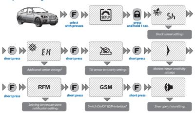
Main system parameters and settings can be changed using LCD remote. To enter the settings menu, select in icon by pressing button and confirm by pressing to button for 1 second. To
