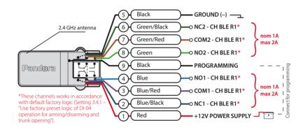
Enter the programing level Nº10.7 - "Pairing an additional device". The LED will light green or red (the red LED means a radio relay has been already paired). · Connect the wire 5 (GROUND) to a grounded spot of a
