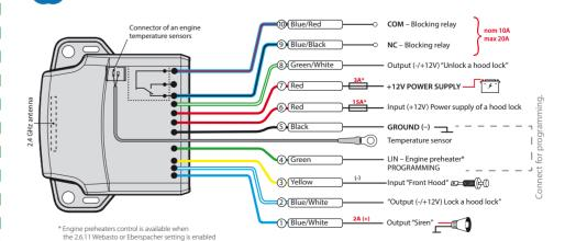
Enter the programing level №10.6 – "Pairing an engine compartment module". The LED will light green or red (the red LED means a module has been already paired).
