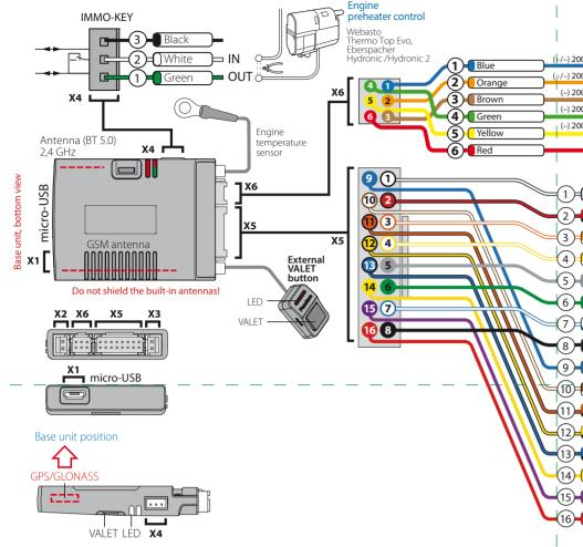
GPS/GLONASS antenna should be placed in the top for better reception of the satellite signal
