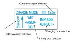
**Charging type selection** – select a type of charging: pulse (asymmetric pulse charging) or direct (normal charging). Confirm selection using button "7" (OK).
