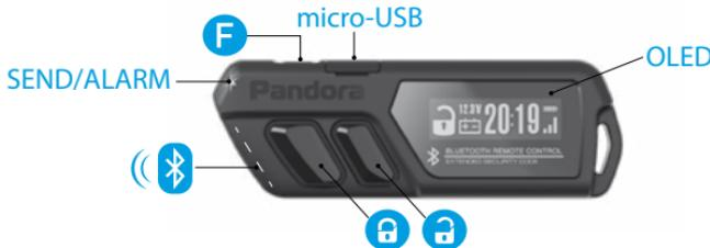
! ALL CONTROL COMMANDS ARE TRANSMITTED VIA RADIO CHANNEL, FOR MAXIMUM EFFECTIVENESS AND RANGE IT IS RECOMMENDED NOT TO SHIELD AERIAL AREA (SEE PICTURE) WITH FINGERS WHEN USING A REMOTE CONTROL.
