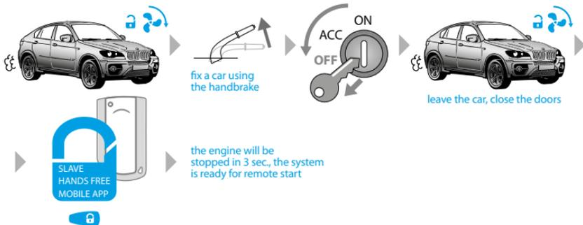
If you are planning to use remote and automatic engine start on a car with manual transmission, before arming you will need to perform following actions:
