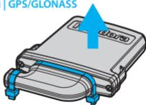
**WARNING!** Do not shield the built-in antennas when installing the system and additional devices. Keep minimum distance of 2 sm between the modules and metal parts.
