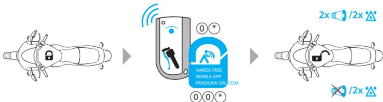
**Clutch lever** – Press the clutch lever when a radio tag is in the coverage zone
