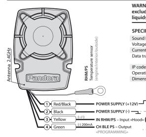
WARNING! The siren must be installed in the places that exclude mechanical damage and ingress of corrosive liquids and water. Do not shield the built-in antenna.
