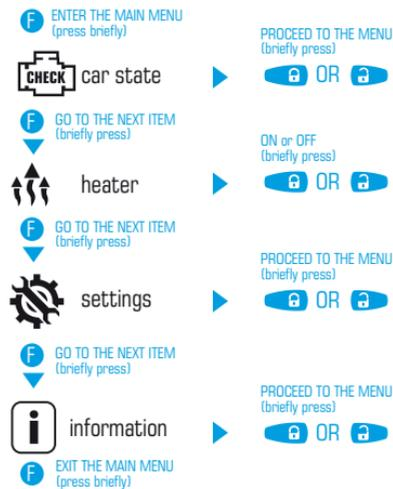
You can manually exit the menu by pressing the **F** button for 1 second. If there are no any actions within 5 seconds, the remote control will exit the main menu automatically.
