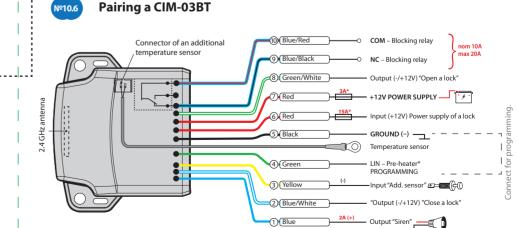
SUPPLY). Connect them to +12V. · If pairing was successful, the LED will light red and the siren/beeper will sound a beep. The system will enter the programming level Nº0.
