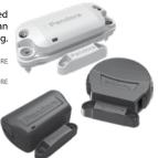
**Movement sensor PIR-100BTM | PIR-100BT** is a wireless device designed to monitor internal volume of a vehicle for thermal movement.
